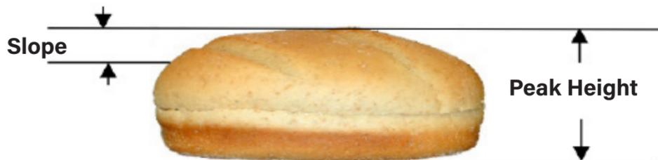
**Profile height calculations** are based on hundreds of individual height values gathered on every product, which leads to a measurement accuracy of  $\pm 0.5\text{mm}$ . **Mean Height** is another common measurement applied to buns.
